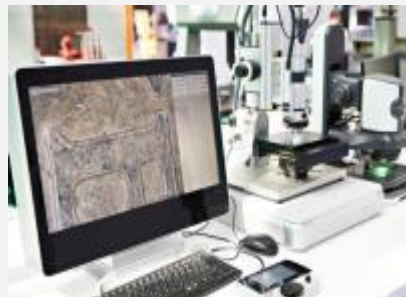
Vicker Hardness tester with Micro Structure Analysing software
